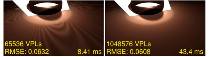
**Figure 11:** Caustics created by highly specular surfaces (roughness: 0.02). A larger number of VPLs has to be generated for higher-frequency BRDFs to reduce the error.
