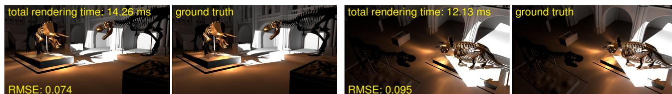
**Figure 1:** Dynamic single-bounce diffuse-to-diffuse and glossy-to-diffuse indirect illumination using 65536 virtual point lights (VPLs) performed on an NVIDIA<sup>®</sup> GeForce<sup>®</sup> GTX 970 GPU (1.47M triangle scene, 1920×1080 screen resolution). Glossy caustics created by GGX microsurfaces are rendered efficiently with our method culling VPLs using random light ranges for GGX reflection.
